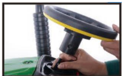
Installing steering wheel
