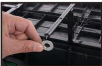
Put on the gasket and then install the wheel
