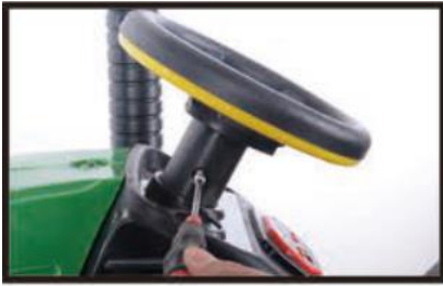
Put on screws and tighten screws
